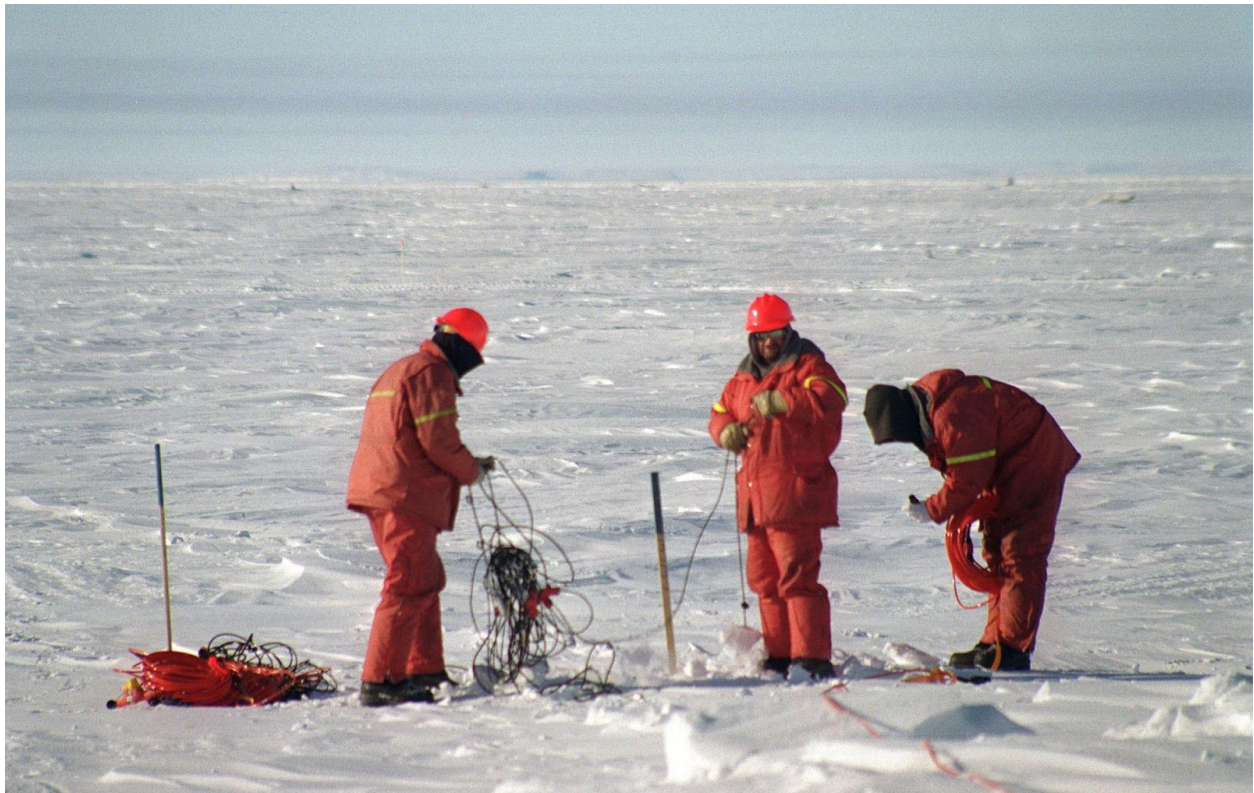
Seismic lines are used to detect natural gas and other underground deposits on the frozen Beaufort Sea. (Tom Cohen / Associated Press)
